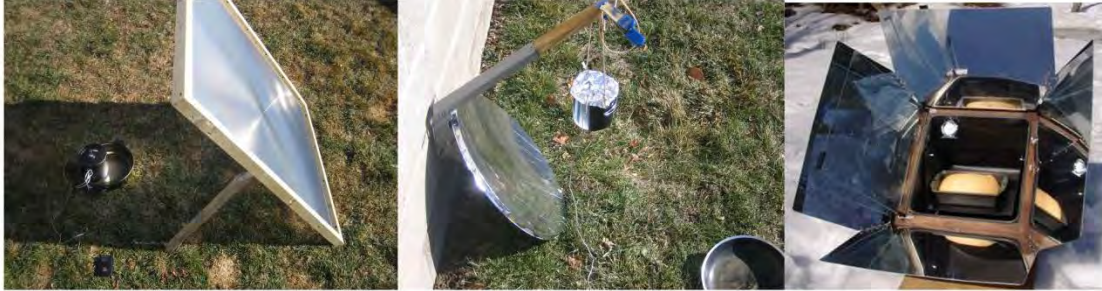
Figure 38 - Cooking with Sunlight. Left: Fresnel lens salvaged from an old projection TV; Middle: Old satellite dish coated with mylar tape; Right: Solar oven from SunOvens.
