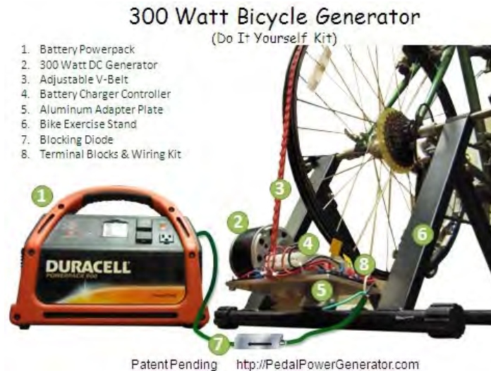
Figure 35 - 300 Watt DIY Human powered generator with a bicycle.
