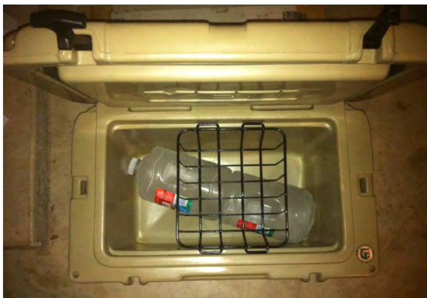
Figure 9 -Inside of a Yeti cooler with 2 gallons of water to act as thermal mass.
